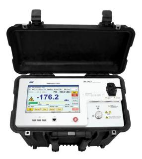
Passive Intermodulation (PIM) is an unwanted mixing effect caused by non-linearity of passive components in the RF path of telecommunication systems. PIM diverts signal energy to other frequencies (spurious signals). This can generate interfering signals that may fall into receiving bands causing serious degradation of system performance.
