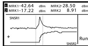
The PULSE mode graph allows the measured waveforms to be shown in a real-time "oscilloscope" format, which can be zoomed or panned as desired.
