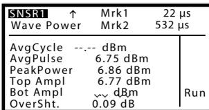
As an alternative to manual cursors, the automatic time gating feature locates the burst start and stop times from the edge transitions, and performs the measurement over a user-defined portion of this time interval.
