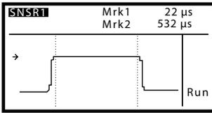
Screen cursors can be easily positioned over the active portion of a single GSM timeslot, allowing measurement of average power and crest factor during this interval.
