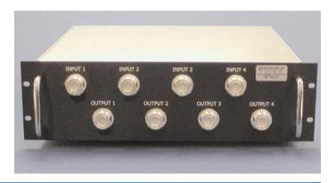
These Combiner Boxes have been designed to meet the special co-siting needs of the wireless market. They are most commonly used to combine up to four wireless carriers in the operating band to single or multiple antenna feeds or distribution cables. In situations where four similar feeds can be utilized, as required in many in-building applications, all four outputs may be used, eliminating the need for terminating unused ports and the 6 dB hybrid loss.
