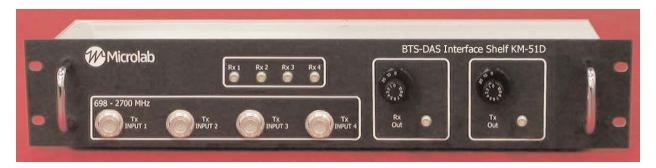
This Signal Conditioner Shelf, suitable for any Tx/Rx signal falling in the 698 - 2700 MHz frequency range, is intended to allow independent level adjustment of the Tx and Rx elements of a wireless signal, when the signal is already split into Tx and Rx paths.
