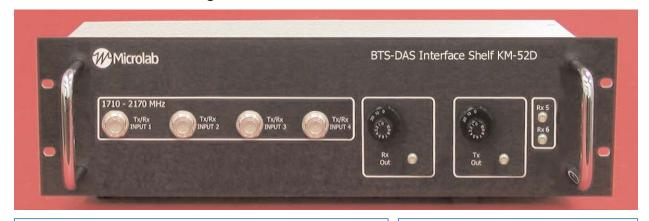
This Signal Conditioner Shelf, KM-52D is designed to interface four Tx/Rx signal blocks within the frequency band 1710-2170 MHz, with a simplex DAS system. It allows independent level adjustment of the Tx and Rx elements of a wireless signal, when the signal is already split into Tx and Rx paths.
