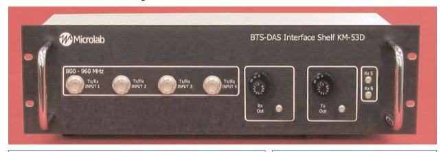
This Signal Conditioner Shelf, KM-53D is designed to interface four Tx/Rx signal blocks within the frequency band 800 - 960 MHz, with a simplex DAS system. It allows independent level adjustment of the Tx and Rx elements of a wireless signal, when the signal is already split into Tx and Rx paths.
