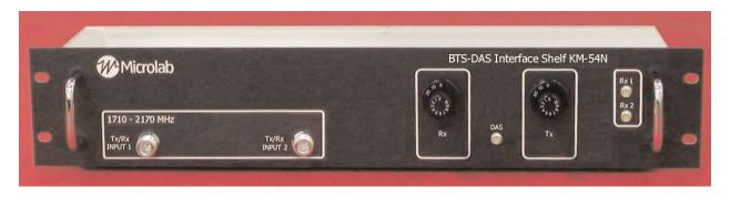
This Signal Conditioner Shelf, KM-54N is designed to interface two Tx/Rx signals within the same frequency bands anywhere in the 800 - 2170 MHz frequency range, with a simplex DAS system. It allows independent level adjustment of the Tx and Rx elements of a wireless signal, when the signal is already split into Tx and Rx paths.
