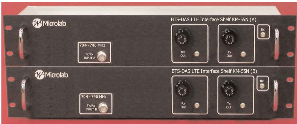
This Signal Conditioner Shelf, KM-55N, is designed to interface the two Tx/Rx signals of an LTE signal in the LTE-700 band, with a dual simplex DAS system. It allows independent level adjustment of the Tx and Rx elements of a wireless signal, when the signal is already split into Tx and Rx paths.
