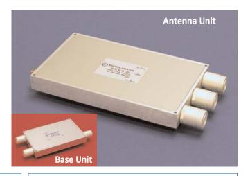
BK-80/90 series is a Diplexer designed for the North American market which allows combination and separation of the signals in 806 - 894 MHz and the 1850 - 1990 MHz wireless bands. To minimize band inter-reaction, the inputs are well isolated and have minimal insertion loss over their respective frequency bands. The design ensures low passive IM.
