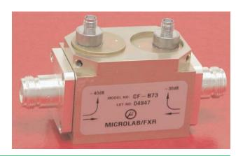
Microlab/FXR loop couplers are set-and-lock devices that provide precise coupling values over customer specified frequency ranges and excellent unit-to-unit tracking. Air dielectric main lines provide the extremely low insertion loss required to handle high power levels. They are available in single and dual units for use over bandwidths of 15% or less, anywhere in the 200 to 3000 MHz frequency range.
