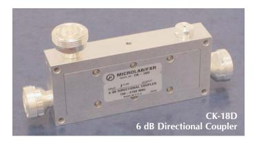
The CK-10 series of Directional Couplers is a tapered stripline design for indoor applications covering from 700 to 2,700 MHz (close to specification from 500 to 3,000 MHz). Units couple off a defined fraction of signal with minimal reflections or loss. Each model is available with or without an internal 4th. port termination.
