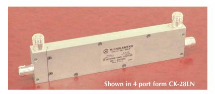
Microlab/FXR CK-20N series, Directional Couplers, is a quarter wave, air-line design for indoor Tetra applications 380 - 520 MHz, and useable down to 150 MHz. Units couple off a defined fraction of signal with minimal reflections or loss.
