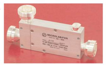
Microlab/FXR CK-30D series, Directional Couplers, is a quarter wave, air-line design for indoor and outdoor applications covering all cellular bands to 2200 MHz. Units couple off a defined fraction of signal with minimal reflections or loss.
