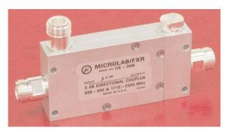
Frequency Ranges: 806 to 960 MHz and 1710 to 2200 MHz VSWR: 1.20:1 max., all ports Dissipative Loss: 0.1 dB max. (Main Line) Power Handling: 200 W avg., 3 kW peak\* 25 dB min., < 1990 MHz Directivity: 23 dB min., > 1990 MHz
