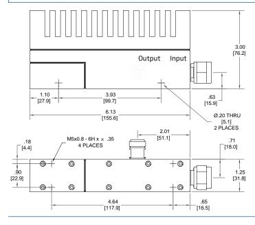
Frequency Range<sup>†</sup>: 698 -1400 & 1650-2700 MHz Impedance:  $50\Omega$  nominal PIM (Intermod): <-150 dBc (+43dBm x2) <-160 dBc typical Peak Power: 3 kW Environment: -35° to +75°C\*, IP67 Finish: **RoHS Compliant** Body Passivated aluminum Connectors: Triplate, N Mounting: Optional brackets or using tapped holes Weight, nominal: 32 oz, (0.91 kg) \*Derate max power by -1.2%/°C above 55°C †Unit non operational in range 1.40 -1.65 GHz
