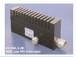
Microlab AY series of fixed Coaxial Attenuators is a tapper based design for medium power wireless applications where low, guaranteed PIM performance is critical. Units are sealed to meet IP 67 for indoor or outdoor applications. The design is exceptionally rugged, and negligibly affected by changes in ambient temperature. Low PIM Attenuators with higher power ratings from 100 to 150W are available as the AZ series.
