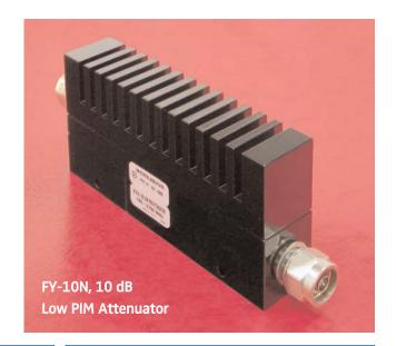
Microlab FY series of fixed Coaxial Attenuators is designed for medium power wireless applications where low, guaranteed PIM performance is critical. Standard model is unidirectional with a conventional male input feeding to a female output on the opposite face of the attenuators. Other connector configurations are available to special order.
