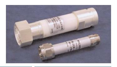
These DC Blocks are used to prevent the flow of direct current and low frequency current surges along the inner and outer conductors of a transmission line, while permitting the unimpeded flow of RF signals. Applications include the blocking of current surges in subway tunnels and at antenna sites during lightening storms. HR-21 series is similar except only the outer conductor is blocked.
