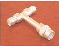
Microlab Model D2-D6 Power Splitters have been designed to evenly split high power signals with minimal reflections or loss. Units may also be used as low loss coherent combiners provided all inputs are both amplitude and phase coincident. Designed with only a few solder joints and an air dielectric, the loss has been minimized and reliability enhanced.
