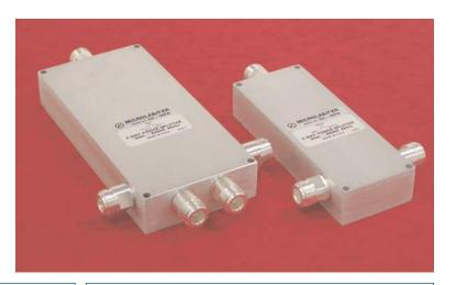
This Dx-49FN series of 2 & 4 way Wilkinson style Power Dividers covers the ultra broad band of 350 - 6,000 MHz using a multi-section microstrip design.
