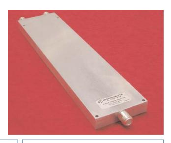
This 2 way Wilkinson style Power Divider covers the ultra broad band of 70 - 2,700 MHz using a multi-section stripline design using an air dielectric for lowest possible loss. The ultra wide bandwidth and reasonable output isolation of this product can eliminate the need for multiple cable paths in the design of distributed antenna systems.
