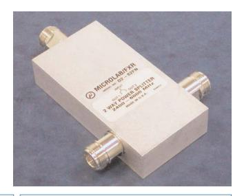
This series of Wilkinson style Power Dividers covers all the WLAN bands using a multi-section stripline design with an air dielectric for lowest possible loss.
