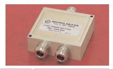
Microlab Power Dividers Models D2-65FN and D2-65MN (with male input) are 2 way Wilkinson style Power Dividers, designed for medium power applications up to 50W where output isolation is preferable over lowest possible loss. The wide frequency range of this design allows use with multiband antennas and leaky cable systems.
