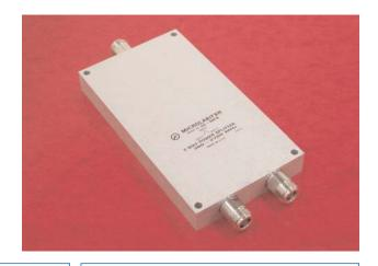
Microlab Model Dx-68FN series of Wilkinson style Power Dividers has been designed for low power applications where output isolation is preferable over lowest possible loss. The wide frequency range of this design allows use with multiband antennas and leaky cable systems.
