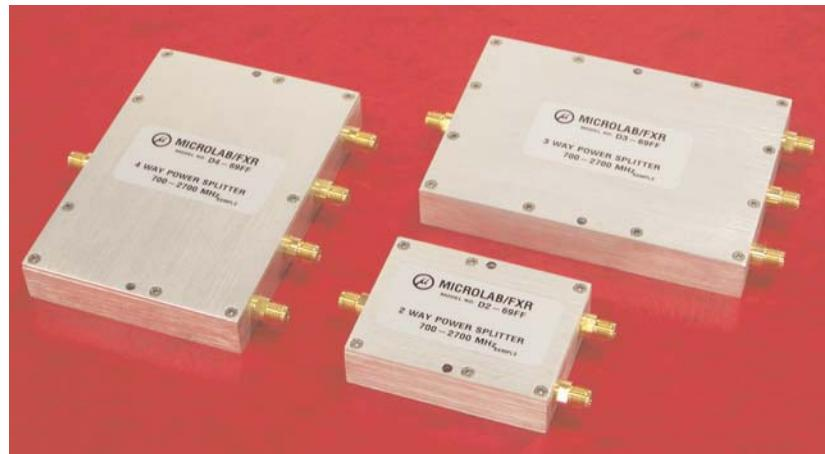
Microlab Model Dx-69FF series of Wilkinson style Power Dividers has been designed for low power applications where output isolation is preferable over lowest possible loss. The wide frequency range of this design allows use with multiband antennas and leaky cable systems.
