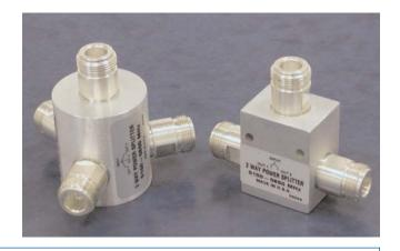
These 2 and 3 way Wilkinson style Power Dividers have been designed using an air dielectric for minimal loss. They have been designed for 5 - 6 GHz Unlicensed National Infrastructure band applications, which includes upper band WiMAX and the 5.8 GHz Wi-Fi/ISM band. (01/09)
