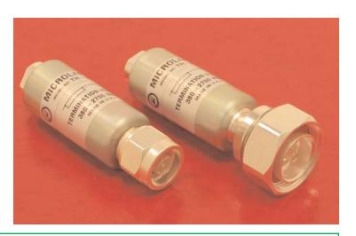
Microlab/FXR TH-2 series of Hybrid Terminations are low power, coaxial loads, which in standard form have a  $220\Omega$  resistance at DC and a  $50\Omega$  from 380 to 2,700 MHz.
