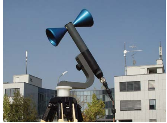
Measurement with 9170 Biconical Antenna
