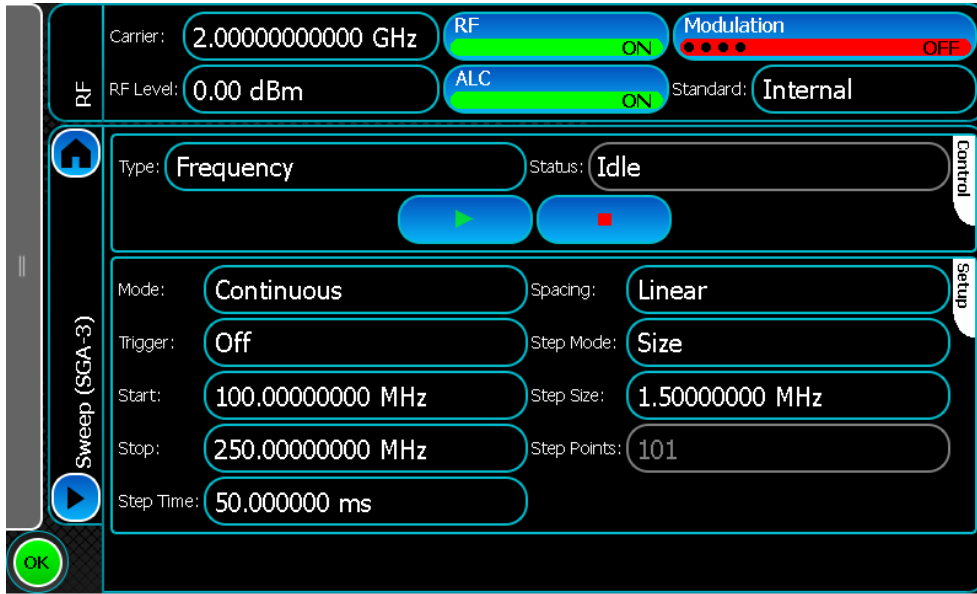
Typical frequency sweep set-up
